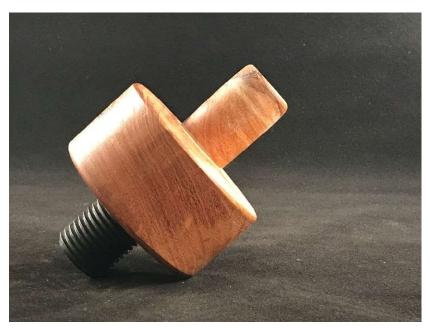
This jig has become a useful addition to my shop. I use it as an extra hand when finishing bowls and when filling voids with turquoise or epoxy. And all it cost was about \$25, and an hour turning the mesquite portion of the jig.
