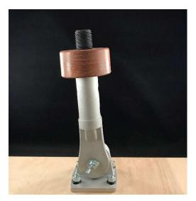
The jig consists of a bracket that can be purchased from Home Depot, a 2" long threaded rod 1-1/4" 8 TPI, and a piece of mesquite that was turned to fit in the bracket and accept the threaded rod. The bracket can rotate thru 180 degrees, the mesquite piece can rotate 360 degrees. A chuck or faceplate fits on the exposed threaded rod, as seen below:
